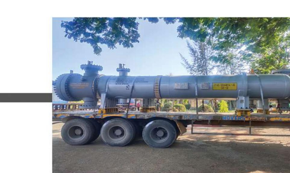
Our Screw Plug Heat Exchangers (SRX<sup>™</sup>) are known all over the world for patented Shrink Ring technology used for high pressure, high temperature, corrosive, hazardous and dirty service applications within Hydrocrackers, Hydrotreaters and other Desulphurisation units of a refinery.
