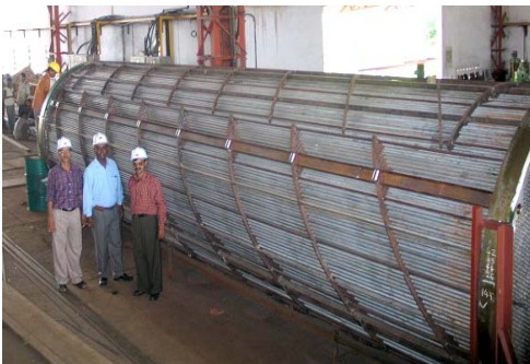
WORLD'S LARGEST HORIZONTAL HELIX TUBE BUNDLE (5500 TUBES) IS READY
